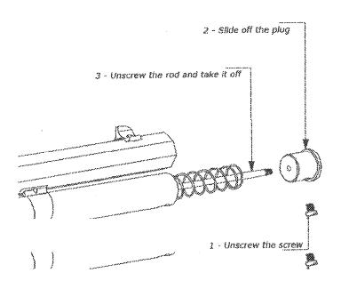
When the rod has been taken off, replace the plug in its seat. In Take Down version there are two screws to disassemble.
