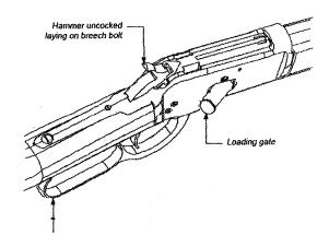
With the muzzle pointed in a safe direction, the lever must be completely closed to load the magazine. The hammer must not be cocked. With thumb securing bummer pull the trigger and slowly lower the hammer.
