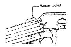
the firing pin pull it slightly rearward until you hear the half cock click. This is the original safety position, if you pull the trigger, the hammer will not be released. To start shooting you have to pull the hammer back to the full cock position. Now you're ready to shoot.
