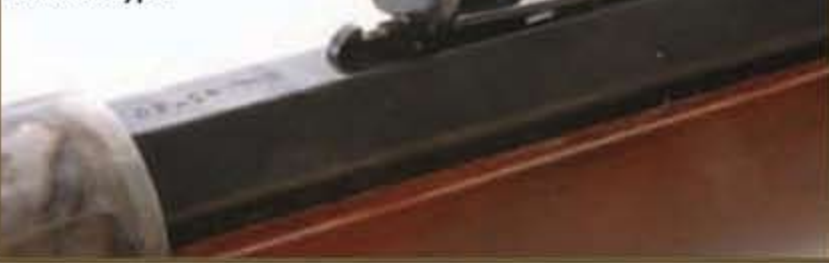
The rear sight on the new Cimarron/Uberti Model 1876 is a traditional buckhorn type.
