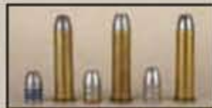
The three loads test fired in the Cimarron/Uberti Model 1876 .45-60 included (from left) 300-grain Oregon Trail FN with loaded round, 324-grain RCBS 45-300FN with loaded round and 336-grain Lyman 457122 with loaded round.
