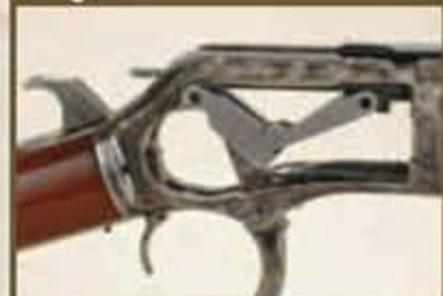
The toggle-link system of locking the breech of a Model 1876 is not strong, but will suffice for the modest pressures generated by proper .45-60 loads. This is certainly no candidate for magnum pressures.
